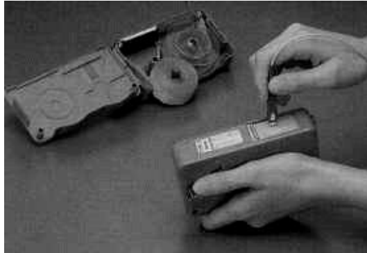
Figure16: Evertz recommended fiber optic cable cleaner made by Cletop
